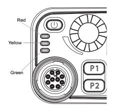
Blinking yellow - Radio is scanning for activity or receiving a Call Alert.
