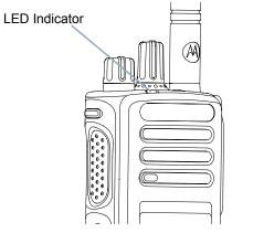
**Blinking red** – Radio is transmitting at low battery condition, receiving an emergency transmission or has failed the self-test upon powering up.
