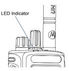
**NOTE:** The LED lights up solid green while the radio is transmitting and double blinks green when the radio is receiving a privacy-enabled call.
