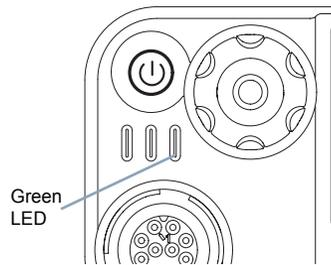
**NOTE:** The green LED lights up while the radio is transmitting and double blinks when the radio is receiving a privacy-enabled call.
